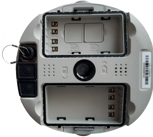
Figure 2-3: Battery compartment door removed
