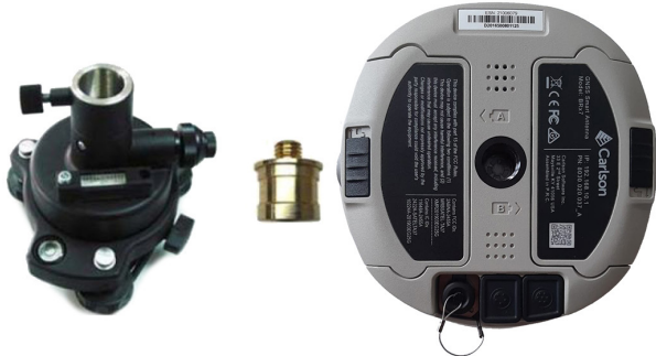
Figure 2-6: Installing BRx7 on a tribrach
